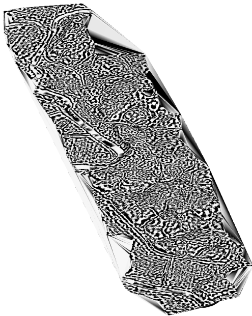
Figure 7: The signed errors for the Serpent Mound dataset and Wendland's RBF \phi_{3,1} with \alpha = 0.01 : the positive error is colored white and the negative error is colored black.
