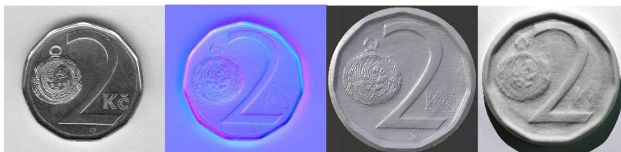
**Fig. 5.** Results of a '2 Kč' coin. Left to right: original, normals, reconstruction, 3D print.
