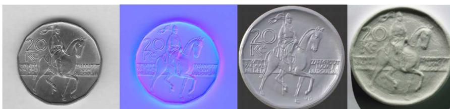
**Fig. 6.** Results of a '20 Kč' coin. Left to right: original, normals, reconstruction, 3D print.
