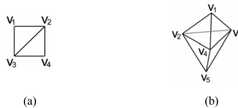
Figure 2. Each diamond is composed of two neighboring simplicial mesh cells, sharing a common face. Reference diamonds are depicted for 2D (a) and 3D (b) simulation mesh
