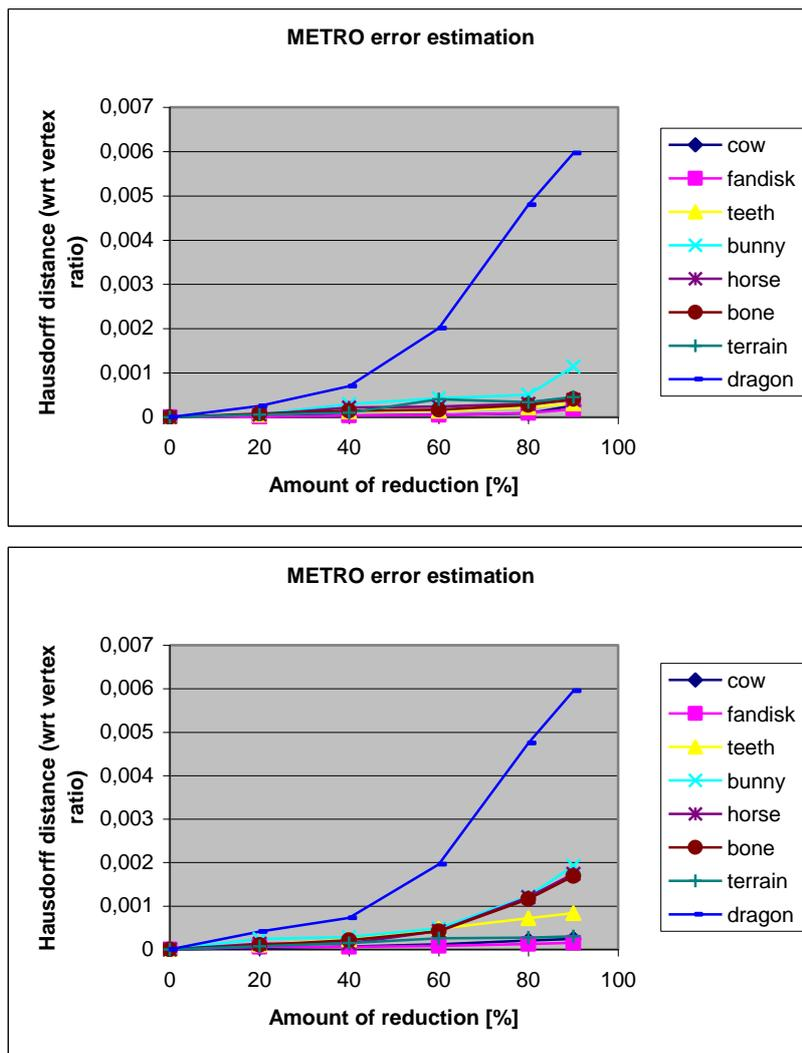
Fig. 16: Approximation error for certain LOD for approaches with (upper) and without (lower) memory.
