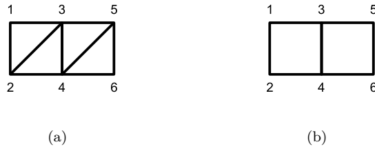
FIG. 1.1. An example of sequential triangle strip 1.1(a) and a sequential quad strip 1.1(b).
