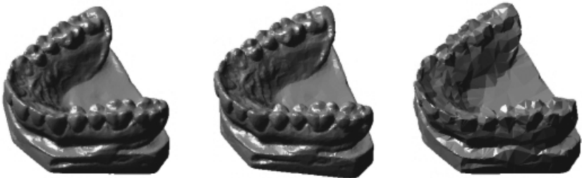
Fig. 7. A teeth model (courtesy Cyberware) at different resolutions; the original model with 58,328 triangles on the left, reduced to approx. 29,000 triangles in the middle and 6,000 triangles approximation on the right
