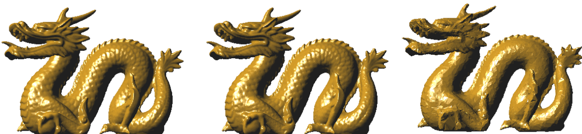
Figure 10: A dragon model (courtesy GaTech) at different resolutions; the original model with 871,414 triangles on the left, reduced to approx. 430,000 triangles in the middle and 87,000 triangles approximation on the right.
