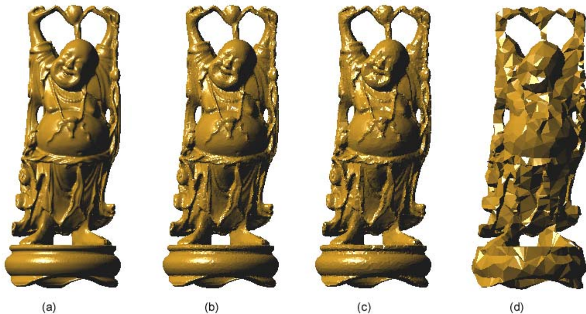
Figure 8: The Happyb model (courtesy GaTech) at different resolutions; the original model with 1.087.716 triangles (a), reduced to 105.588 triangles (b), 52.586 triangles (c), 10.974 triangles (d).
