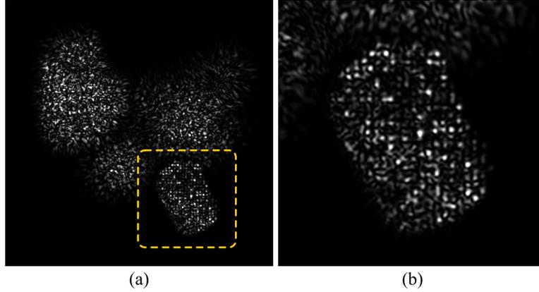
Figure 4.31: (a) A numerical reconstruction of the scene “Primitives2” using an optical field calculated using the frequency masking and (b) an enlarged detail of the reconstruction. Notice the structure that is present in the detail. The reconstruction focuses the cylinder at 8.0 mm.
