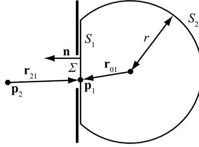
Figure 2.3: The screen and the volume  $S$  used for derivation of the Kirchhoff formulation. [Goo05]
