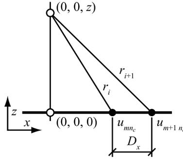
Figure 3.6: A setup used by a diffraction scheme from Eq. (3.3). A sample at  $(0, 0, z_0)$  contributes to samples  $u_{mn_c}$  and  $u_{m+1 n_c}$ , where  $n_c = \text{const.}$  [YIO00]
