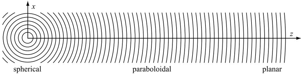
Figure 2.1: Relation between the spherical wave and the planar wave as seen through a small window.
