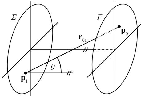
Figure 2.7: A setup used by the Fresnel/Fraunhofer approximation. [Goo05]
