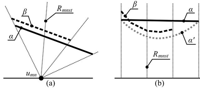
Figure 5.2: (a) A cross-section of two planes sampled by rays originating from the sample  $u_{mn}$  and (b) a cross-section of the same setup deformed to fit the rasterizer. While the plane  $\alpha$  consists of a single triangle, the plane  $\beta$  consists of multiple triangles. As a consequence, a visibility error occurs in (b). The surface  $\alpha'$  represents the plane  $\alpha$  deformed accurately.
