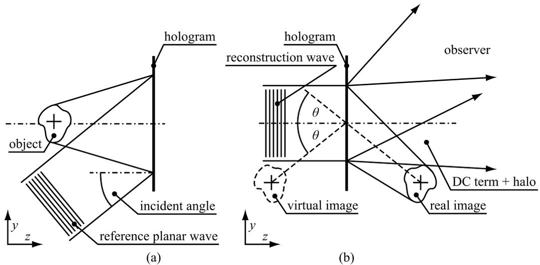
Figure 2.11: (a) An off-axis hologram recording setup and (b) a reconstruction. The angle  $\theta$  represents an incidence angle of the planar reference wave from the hologram. [Har96]
