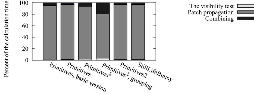
Figure 4.34: A distribution of computational time between steps of Alg. 2. If not noted otherwise, all results we measured using the frequency masking.
