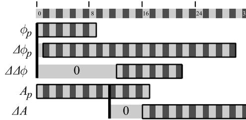
Figure 5.9: Estimated bit ranges necessary to evaluate the differential scheme Eq. (5.12). The thick vertical lines show locations of decimal points.
