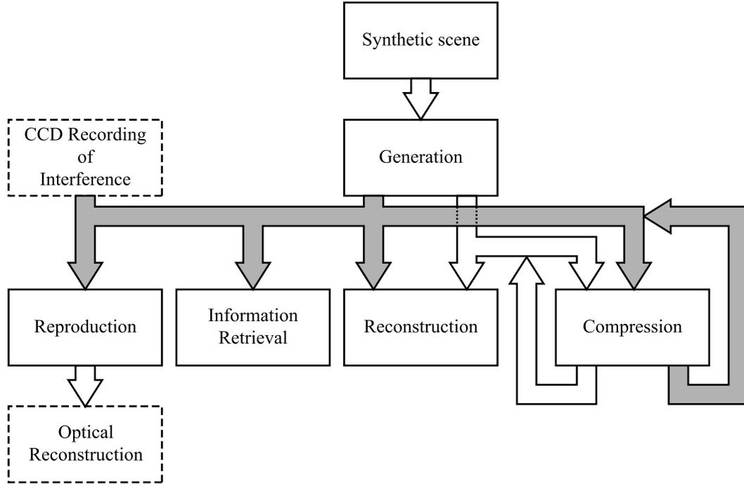
Figure 3.1: Digital holography areas and their relation in a context of this work. The dashed boxes belong to optical holography. Lines between boxes represent data transfer: white lines represent an optical field, greyed lines represent an interference pattern, i.e., a hologram.
