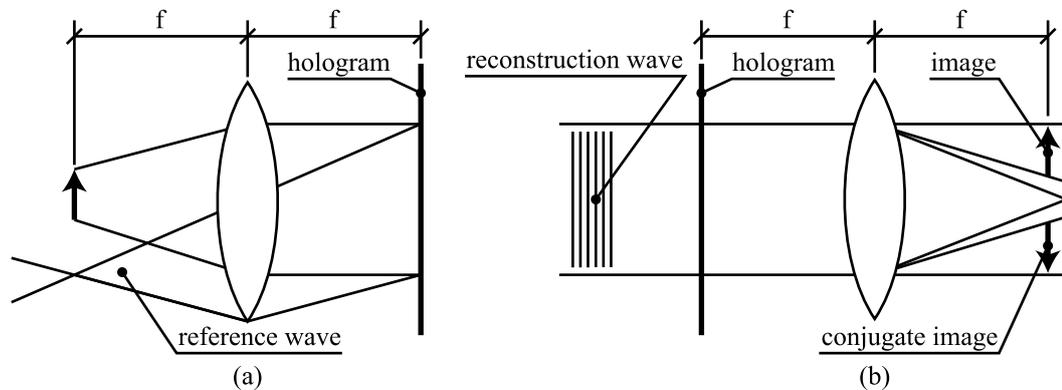
Figure 2.12: (a) A Fourier hologram recording setup and (b) a reconstruction. The distance  $f$  is a focal distance of the lens. [Har96]
