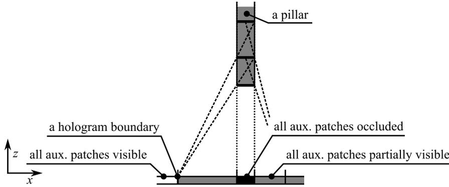
Figure 4.52: Partially occluded auxiliary patches. Decreasing the angle between a direction of a ray and the normal of the plane  $\kappa$ , the dashed lines show the first ray that hits an auxiliary patch from the edge of the hologram.
