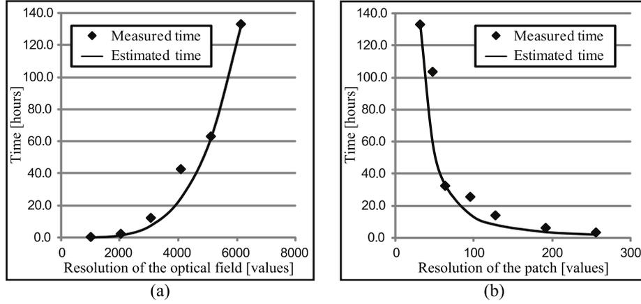
Figure 4.19: Time measurements of our method for the scene “Primitives<sup>‡</sup>”. (a) The patch resolution is constant and both the sampling step and the resolution of the optical field differ. (b) Both the sampling step and the resolution are constant and the patch resolution differs.
