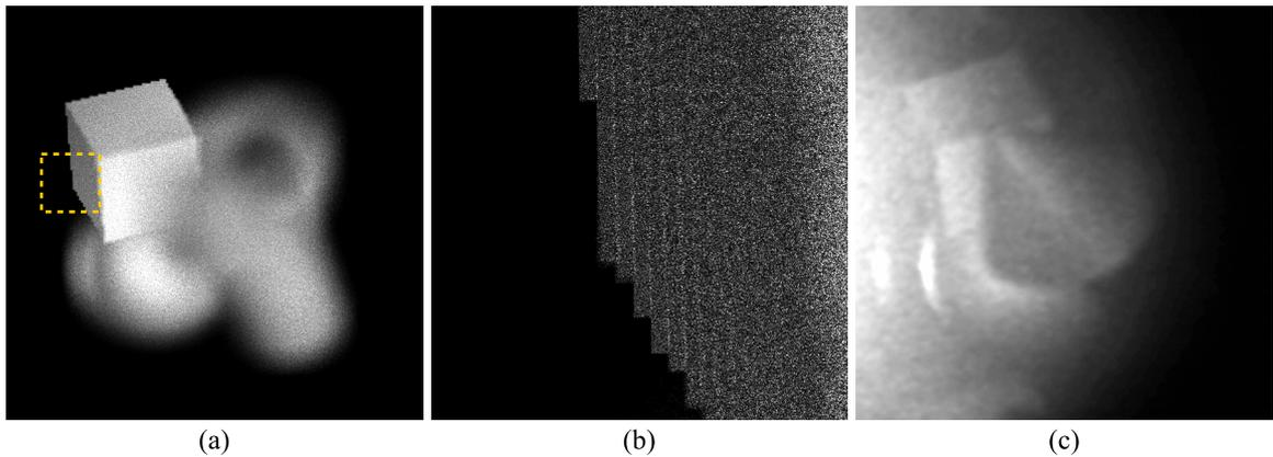
Figure 4.14: (a) A numerical reconstruction of the scene “Primitives<sup>‡</sup>” focused at the cube (0.5 m). The reconstruction uses a propagation in the angular spectrum without a pinhole and a lens. (b) An enlargement of the dashed rectangle showing artifacts in a form of vertical lines. (c) An optical reconstruction focused on the cube. Notice that the artifacts has no influence on the optical reconstruction.
