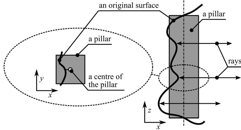
Figure 4.53: Obtaining intensity of an auxiliary patch from known location of the auxiliary path inside a pillar.
