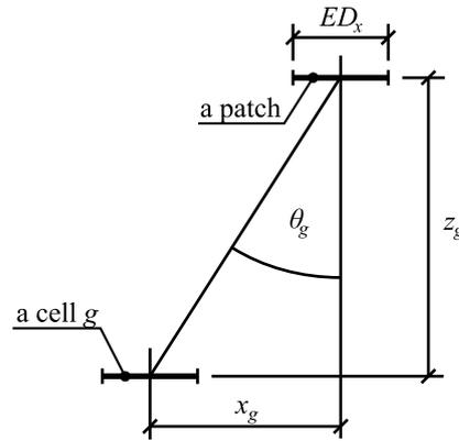
Figure 4.26: A patch and a cell including distanced used by the presented acceleration approach.
