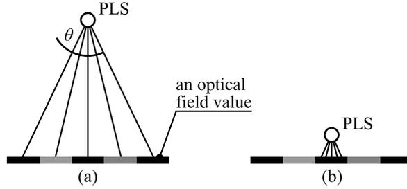
Figure 4.23: (a) PLS contributing to all optical field values and (b) PLS that is too close to contribute to any value but the only the middle. If had been contributing to all samples, it would have created aliasing. The angle  $\theta$  denotes a maximum angle that does not lead to an aliasing.
