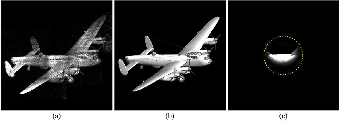
Figure 4.8: (a) An optical reconstruction of a virtual scene with a constant phase on its surface. (b) A numerical reconstruction of the same scene and (c) a numerical reconstruction using an aperture. Notice the missing part of the object due to the pinhole. The dashed circle shows boundary of the aperture.
