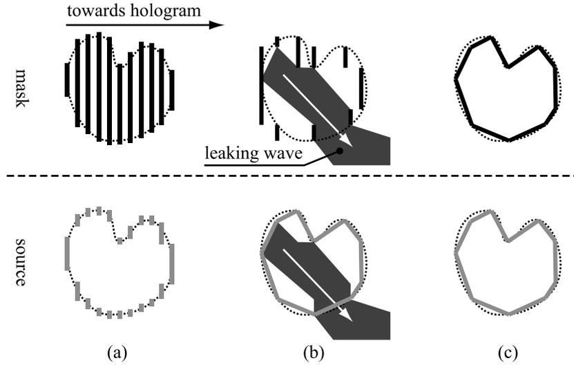
Figure 3.5: A visibility solution for wave-based methods is based on set of masks and corresponding patches of sources. (a) Layered holograms uses parallel planes to slice the scene, (b) the silhouette approximation combines parallel masks with titled sources but suffers from wave leaking, and (c) an exact solution requires frequent rotation of the optical field.
