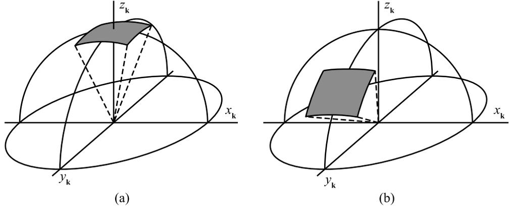
Figure 2.6: (a) All possible wavevectors with  $z_k^2 > 0$  form a hemisphere in the angular spectrum. (b) A rotation of the spectrum rotates a hemisphere. The greyed part of the hemisphere in both (a) and (b) represents the same subset of wavevectors.
