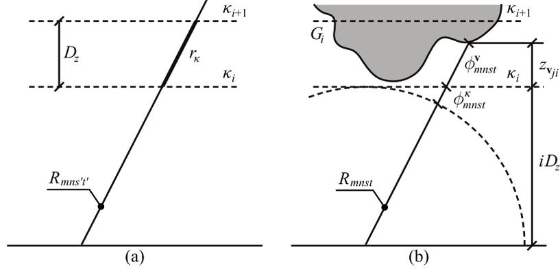
Figure 5.5: (a) Evaluation of the longest distance  $r_\kappa$  and (b) decomposition of the distance including corresponding phase shifts  $\phi_{mnst}^v$  and  $\phi_{mnst}^\kappa$ . The longest distance is computed from  $D_z$  and the extreme ray  $R_{mns't'}$ .
