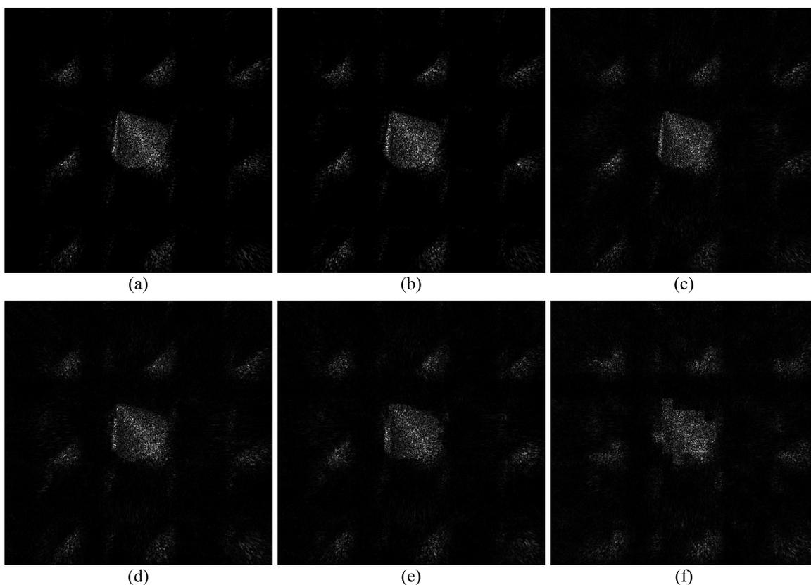
Figure 4.16: An numerical reconstruction of the scene “Primitives” focused at the cone (6.0 mm). The optical field was calculated using a patch size: (a)  $8 \times 8$  samples, (b)  $16 \times 16$  samples, (c)  $32 \times 32$  samples, (d)  $64 \times 64$  samples, (e)  $128 \times 128$  samples and (f)  $256 \times 256$  samples. Notice the coarseness of cone edges when the size of the patch increases.
