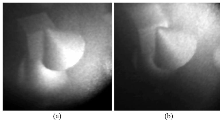
Figure 4.13: An optical reconstruction of the scene “Primitives<sup>†</sup>” focused at the cone. Notice that visibility is solved correctly when viewer changes its location.
