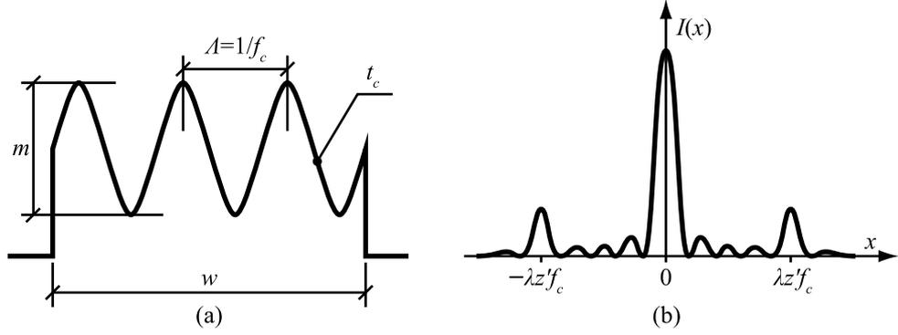
Figure 2.5: (a) The amplitude-modulating function  $t_c$  of a cosine grating and (b) an effect of the cosine grating on a planar wave observed from larger distance. [Goo05]
