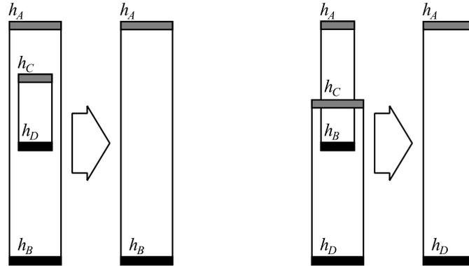
Figure 4.5: Invalid configurations of pillars and corresponding fixes. The black rectangles and gray rectangles denotes front caps and back caps respectively.
