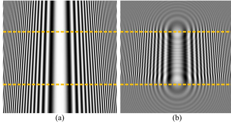
Figure 3.9: (a) A real part of an optical field generated by an infinite line and (b) a real part of an optical field generated by a line segment. The dashed rectangle specifies an area that is considered by the approximation.
