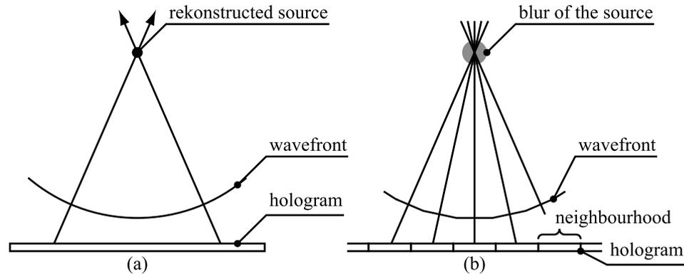
Figure 3.15: (a) A wavefront generated by PLS and (b) a wavefront approximated by a linear function. Notice that (b) is a almost ideal wavefront that lacks all disturbances due to discontinuities between neighbourhoods. [KYY08]
