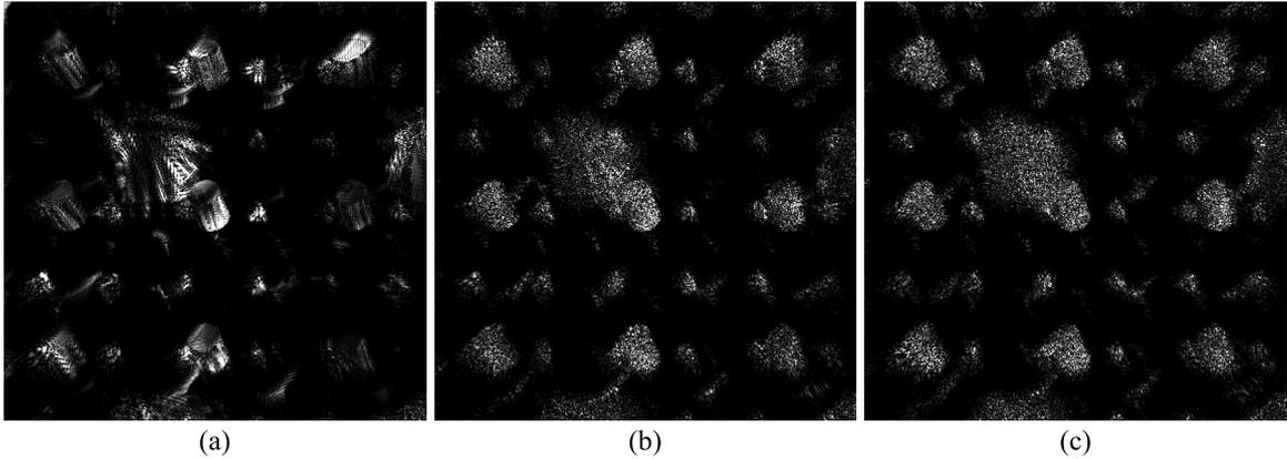
Figure 4.22: Numerical reconstructions from optical fields calculated (a) using a library of a single spectrum, (b) using a library of 8 spectrums, and (c) using a library of 64 spectrums. Notice the intensity variation at the bottom of the cylinder in (a) and (b).
