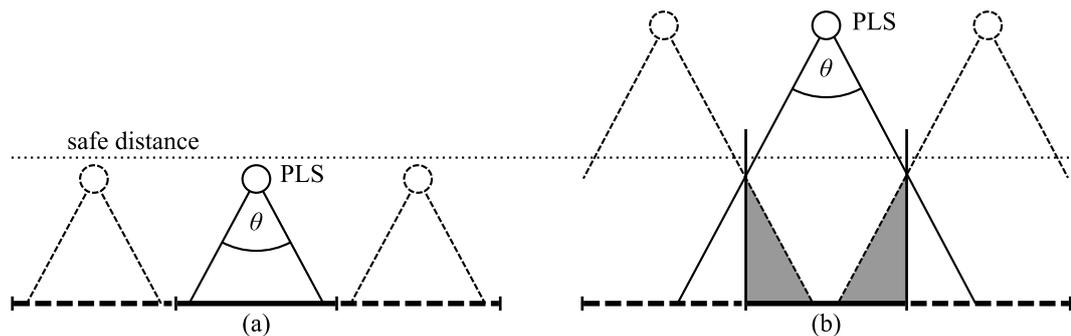
Figure 4.2: An influence of periodicity assumed by DFT on either PLS (a) closer than the safe distance and (b) beyond the safe distance. The angle  $\theta$  is given by Eq. (2.24). The dashed lines indicates a side-effect due to the periodicity, the gray area in (b) shows overlapping of contributions.
