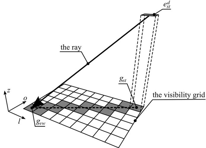
Figure 4.7: A visibility test between the patch  $e_{st}^d$  and the cell  $g_{vw}$ .
