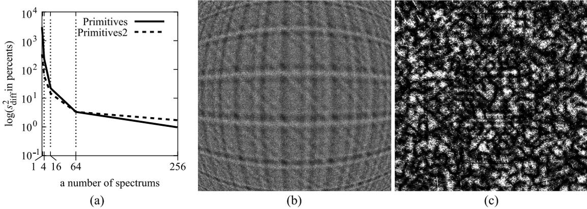
Figure 4.21: (a) A graph showing convergence of sample variance and intensity of samples at the Fraunhofer region for an optical field calculated (b) without the library and (c) with a library of a single spectrum. The graph shows a difference  $s_{\text{diff}}^2$  of a sample variance from a sample variance of a case calculated without the library. A scene in (b, c) is “Primitives”.
