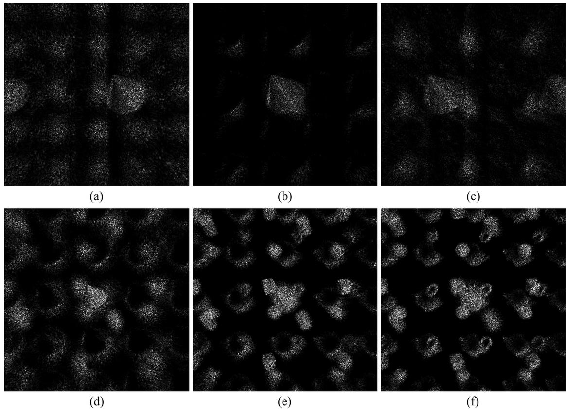
Figure 4.12: (a-c) A numerical reconstruction of the scene “Primitives” focused at the cone. The optical field was shifted horizontally by (a)  $-0.5$  mm, (b)  $0.0$  mm, (c)  $+0.5$  mm. (d-f) A numerical reconstruction of the scene “Primitives2” focused at different objects (different depths): (d) the cone ( $6.0$  mm), (e) the cube ( $10.0$  mm) and (f) the torus ( $14.0$  mm).
