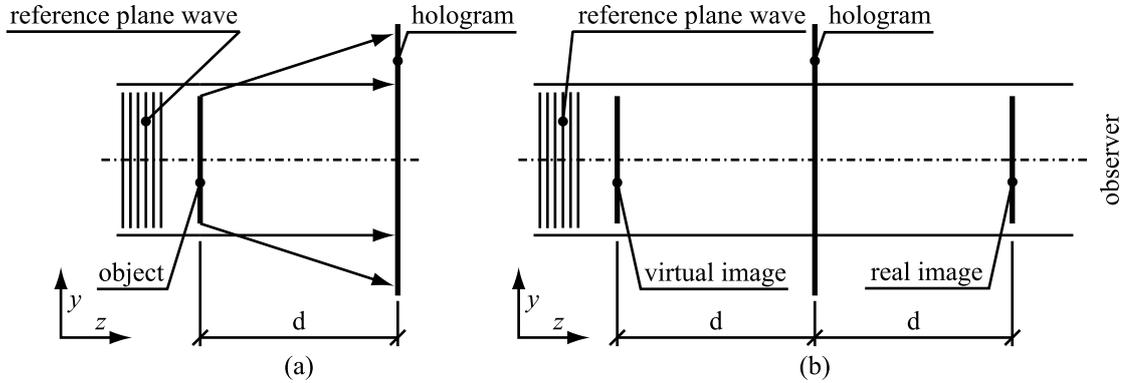
Figure 2.10: (a) An in-line hologram setup for recording and (b) a in-line hologram reconstruction. The distance of the object to the hologram is  $d$ . [Har96]
