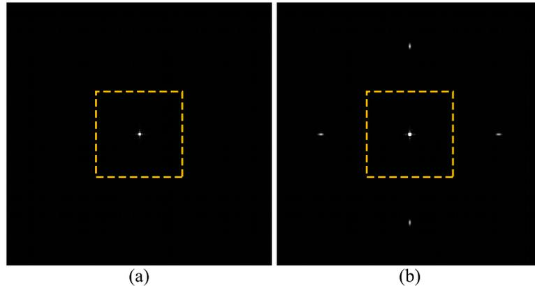
Figure 3.4: A numerical reconstruction of an optical field with added frame of zeros. Optical field was calculated using (a) analytical expression for PLS and (b) propagation of the angular spectrum. Notice the repeating of the pattern due to FFT in (b). The dashed line shows a size of the original optical field.
