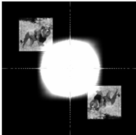
Figure 2.13: A numerical simulation of reconstruction from the Fourier hologram.
