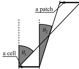
Figure 4.27: Angles used for an estimation of frequency ranges. If we had ignored the diffraction at the edge of the cell, only the plane waves from a range  $[\theta_1, \theta_2]$  would have hit the patch.
