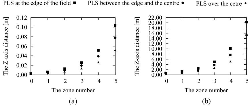
Figure 4.35: A minimum distance for zones calculated using an optical field of  $4,096 \times 4,096$  samples and a sampling step  $D$  of either (a)  $0.5 \mu\text{m}$  or (b)  $7.0 \mu\text{m}$ . In both cases, the wavelength is  $635 \text{ nm}$ .
