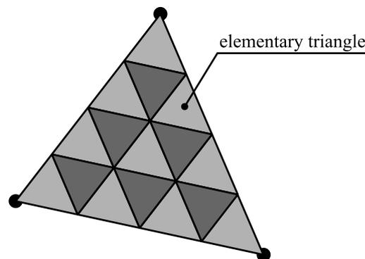
Figure 3.13: A triangle divided into elementary triangles. The division scheme requires two versions of the elementary triangle that are marked by lighter and darker gray. [KHL08]
