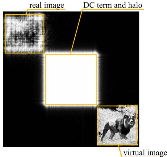
Figure 2.9: An intensity of a propagated optical field. The optical field was formed just after an amplitude-modulating hologram. In this case, the hologram is a recording of sources on a plane with various intensity. The optical field is propagated to a location of the virtual image. At the same time, the real image is out of focus. Notice that this examples present an off-axis hologram.
