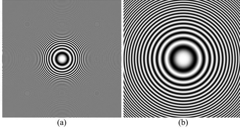
Figure 3.7: A real component of an optical field generated by PLS at (a) a distance  $z_0$  and (b) a distance  $4z_0$ . Notice that additional circles in (a) are a product of an alias.
