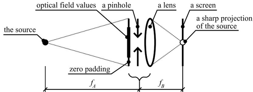
Figure 4.10: A setup used by the numerical reconstruction. The lens, the aperture and the plane with optical field values are located at the same distance from the screen.
