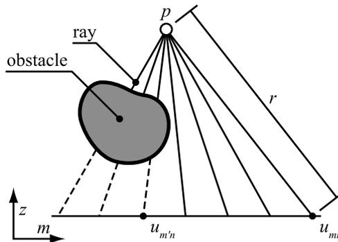
Figure 3.3: Visibility solution of PLS  $p$  using a geometry-based method. While the sample  $u_{m'n}$  does not obtain any contribution from PLS due to the obstacle, the contribution to sample  $u_{mn}$  is proportional to  $\frac{\exp(jkr)}{r}$ .
