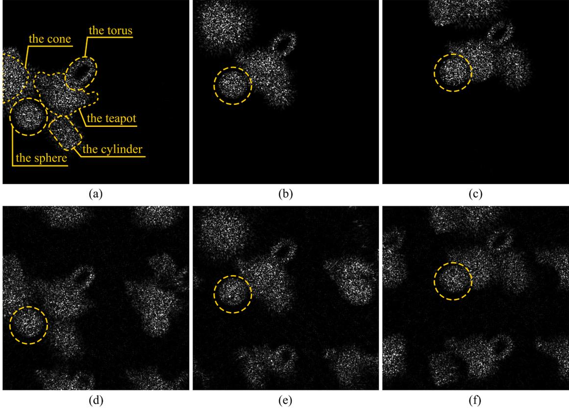
Figure 4.30: Numerical reconstructions of the scene “Primitives2” using an optical field shifted (a,d) by  $(0.7 \text{ mm}, 0.0)$ , (b,e) by  $(0.5 \text{ mm}, 0.5 \text{ mm})$ , and (c,f) by  $(0.0, 0.7 \text{ mm})$ . The optical fields in (a-b) were calculated using the frequency masking, the optical fields in (d-f) were calculated without the frequency masking. All reconstruction focus the sphere at  $12.0 \text{ mm}$ .
