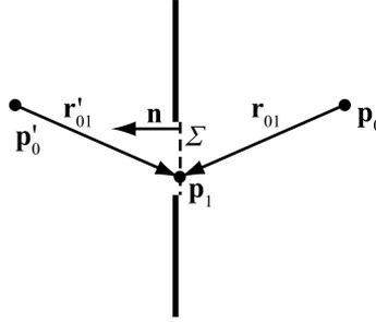
Figure 2.4: A screen and a symmetrical PLS used by a definition of the function  $g$ . The setup is used to derive the Rayleigh-Sommerfeld formulation. [Goo05]
