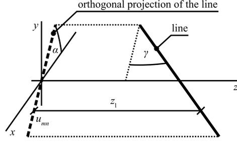
Figure 3.8: A part of an infinite line. An optical field of a line where  $\alpha \neq 0$  can be calculated by rotating an optical field of a line where  $\alpha = 0$ . [FLB86]
