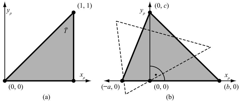
Figure 3.12: Triangle shapes that allow to express the angular spectrum analytically. An angular spectrum of a general triangle can be derived from (a) a special case triangle  $\bar{T}$  [ABMW08] or (b) can be expressed directly using a properly rotated triangle [KHL08]. Dashed line in (b) shows a general triangle prior rotation.
