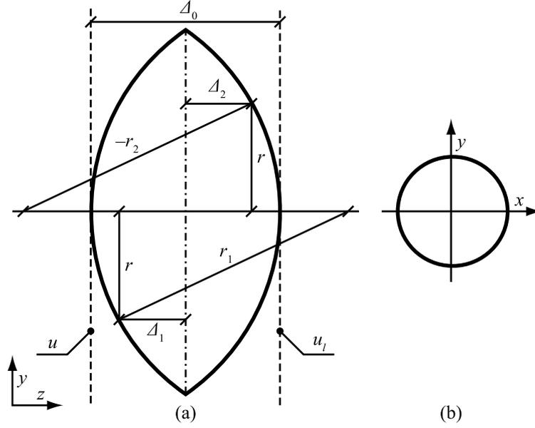
Figure 2.8: (a) A side view of the lens and (b) a front view of the lens. Resulting optical field values  $u_l(\mathbf{p}_1)$  are on the right side of the lens. The input optical field values are on the left side. Notice that the radius  $r_2$  is negative because the waves are assumed to travel from left to right. The radius  $r$  is  $r = (x_{\mathbf{p}_1}^2 + y_{\mathbf{p}_1}^2)^{1/2}$ . [Goo05, SJ05]
