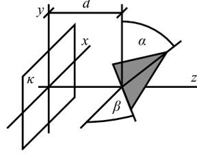
Figure 3.11: A triangle in a table is accessed through three indices: a rotation angle  $\alpha$  about the X-axis, a rotation angle  $\beta$  about the X-axis, and an orthogonal distance  $d$  between the triangle and the plane  $\kappa$ .
