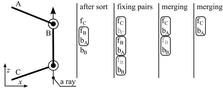
Figure 4.6: An example of a singular case solved by merging of pillars. The processed slice contains an edge from the triangle B that is perpendicular to the plane  $\kappa$  and the ray  $r$  hits the triangle B. Just for purpose of this example, a front cap and a back cap that were generated from the triangle B are denoted as  $f_B$  and  $b_B$  respectively. Greyed caps are added to fix missing member of a pair.
