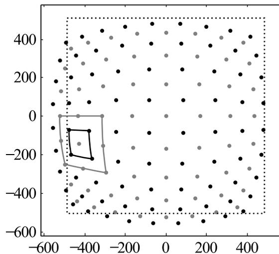
Figure 4.28: Corners of original frequency ranges (gray dots) and corners of used frequency ranges (black dots) including corresponding ranges (solid rectangles). In this case a patch is closer than a distance given by the diffraction condition Eq. (2.24) and therefore some ranges may overlap an edge of the angular spectrum (a dotted rectangle).
