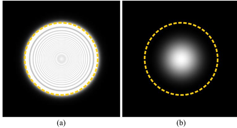
Figure 4.9: Intensity of a plane wave propagated through either (a) a pinhole with sharp edges or (b) an amplitude modulator defined by Eq. (4.6). The dashed circle shows an area where the pinhole function is not zero.
