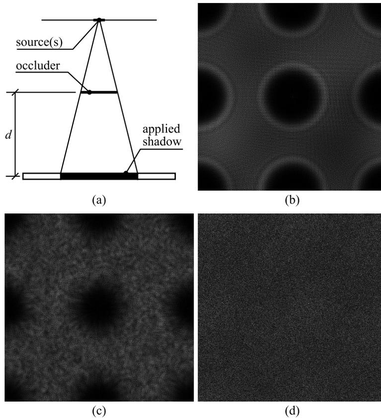
Figure 4.3: (a) The used setup and numerical reconstructions at the distance  $d$ . The source is a patch of (b)  $16 \times 16$  PLS, (c)  $256 \times 256$  PLS, and (d)  $1,024 \times 1,024$  PLS.
