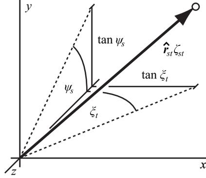
Figure 5.4: Calculation of the correction constant  $\zeta_{st}$ . An orthogonal projection of the directional vector  $\hat{\mathbf{r}}_{st}$  into the Z-axis multiplied by  $\zeta_{st}$  equals to the vector  $(0, 0, 1)$ .
