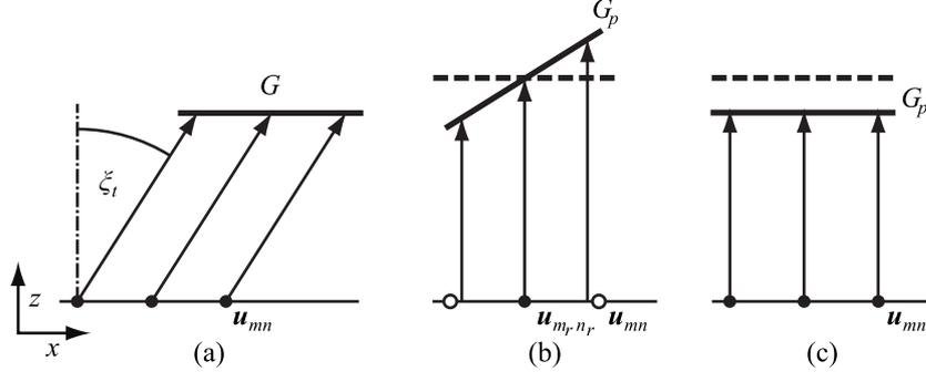
Figure 5.3: Transformations that are able to transform a direction  $\hat{\mathbf{r}}_{st}$  to a vector parallel with a vector  $\hat{\mathbf{r}}_{00}$ . (a) The Mesh  $G$  consist of a single line that can be either (b) rotated or (c) skewed. While rotation leads scaling in all axes, skewing scales only along the  $Z$ -axis. The dashed line shows the desired output.
