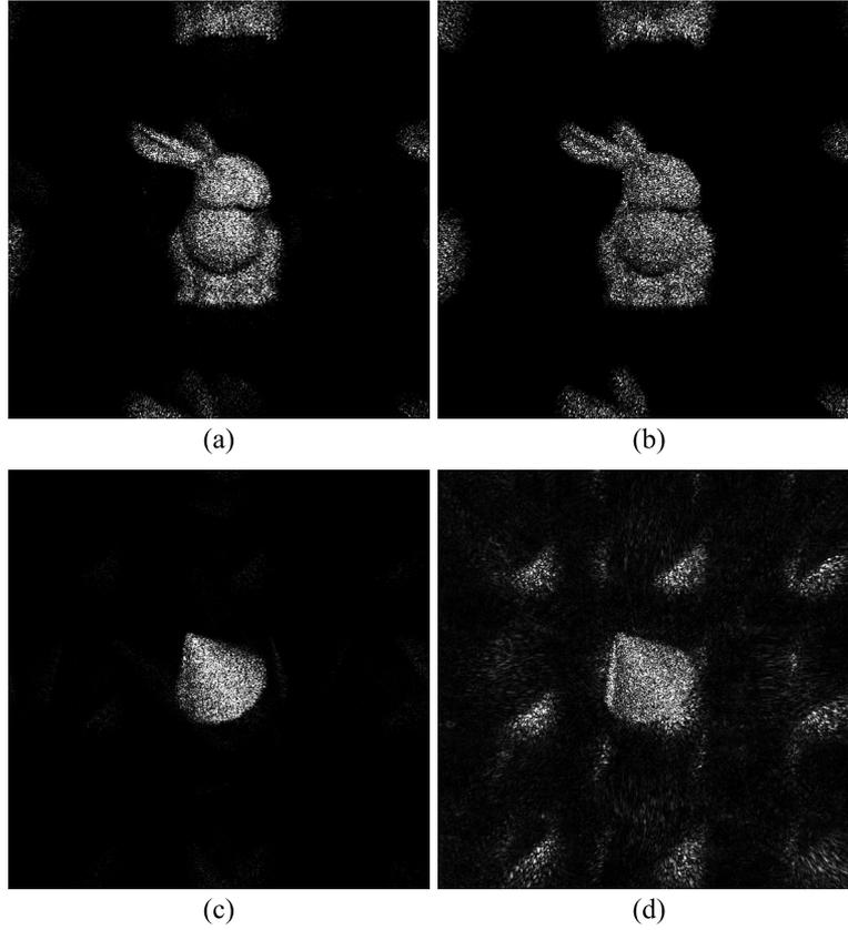
Figure 4.18: (a, c) A numerical reconstruction from optical fields calculated using the AngRay method [JHO08]. (b, d) A numerical reconstruction from optical fields calculate using the proposed methods. Notice the slight deformation of bunny's ear in (b) and a distortion of the cone in (d). Both artifacts are caused by use of patches.
