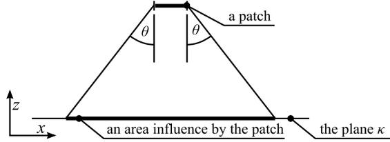
Figure 4.37: A pyramid defined by a patch and a diffraction condition.
