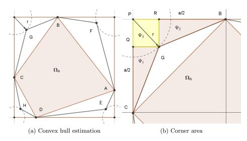
Fig. 2: Axis Aligned Bounding Box and convex polygon
